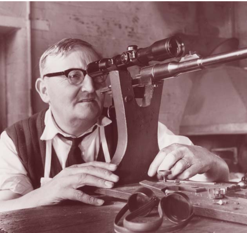
A gunsmith at London's Holland and Holland gun manufacturing company aligns a telescopic sight on the bore of a .244 magnum rifle, December 1962. Holland and Holland has handcrafted firearms since 1835.
