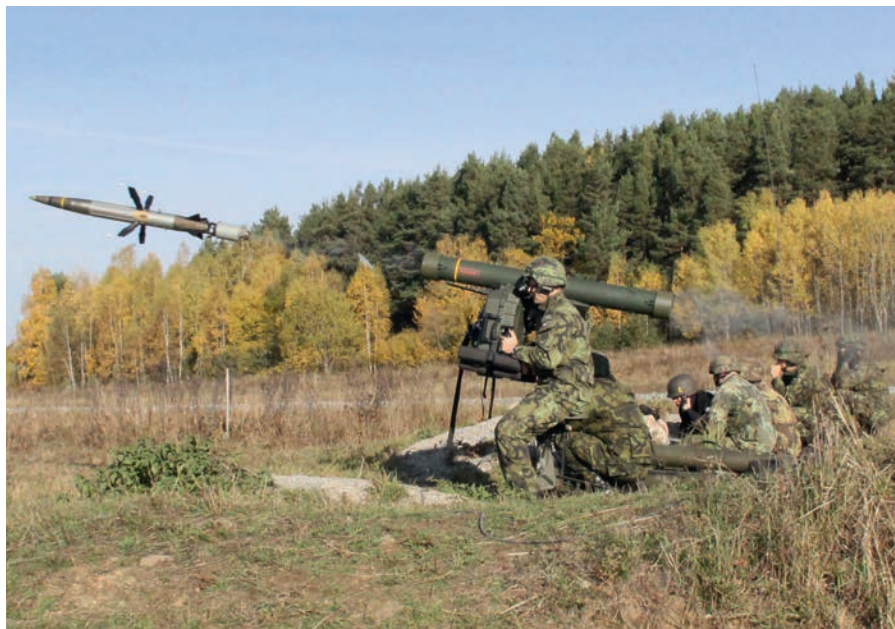
A Swedish Saab RBS 70 NG CREWPADS firing a BOLIDE 'all-target' SAM. Source: Saab
