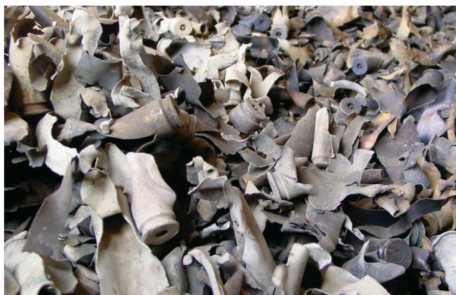
14.5 mm API small arms ammunition scrap following controlled incineration in Albania. © NAMSA
