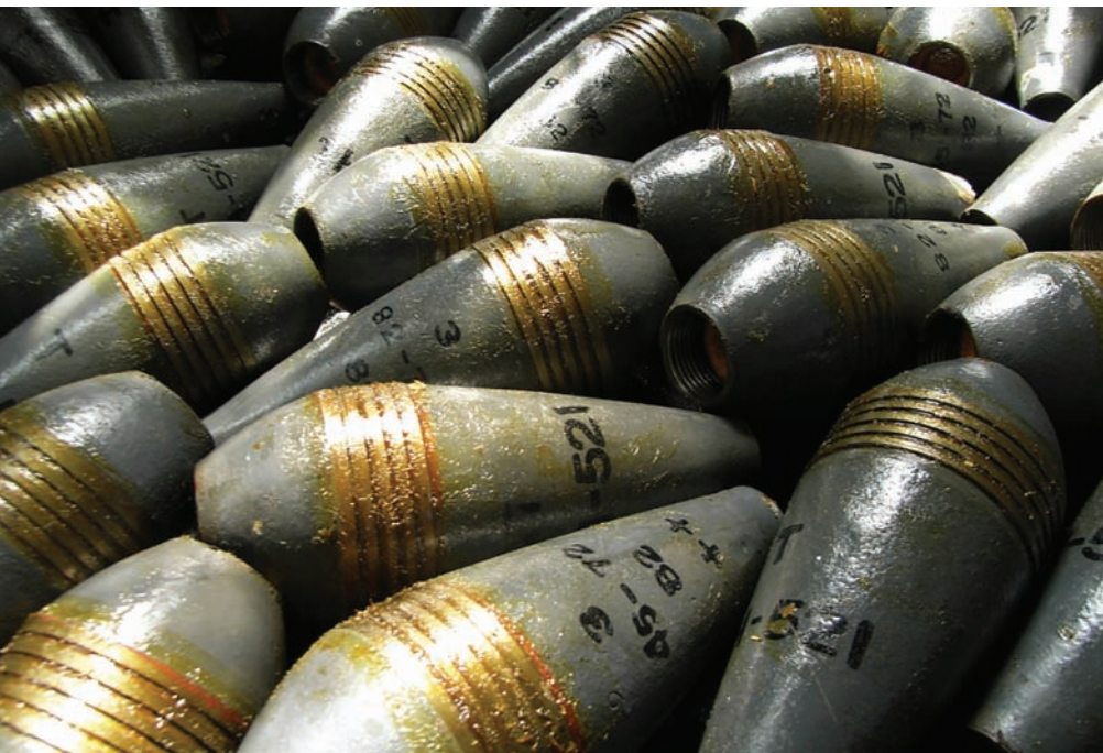
82 mm mortar ammunition scrap awaiting autoclaving, Albania. © NAMSA
