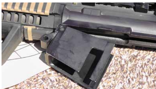
Image 4. The conversion between 7.62 x 51 and 5.56 x 45 includes the quick installation of a magazine adapter.
