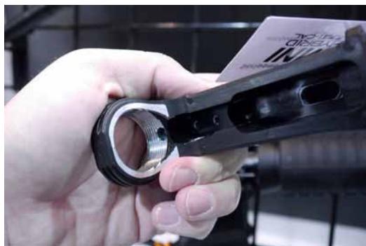
Image 7. A Some polymer lower receivers include a small metal insert to reinforce a particularly weak junction area.
