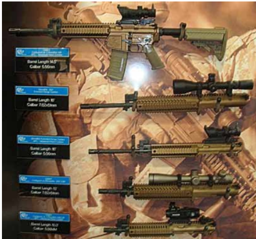
Image 8. Modular weapons offer a wide range of calibre and barrel-length combinations. In the case of the CM901, these combinations are all achieved through swapping the upper receiver on the universal lower receiver. Each upper receiver block can have its own sight/scope mounted, already 'zeroed', ready to be installed.
