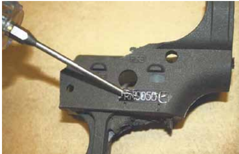
Image 6. A poorly attached metal tag can be removed easily. In the example illustrated by this image, the Firearms Technology Branch of the US ATF tested a sample of a commercial lower receiver against the federal requirements for marking. The serial number was removed easily when a hammer and screw driver were used to peel the sheet off the metal insert. This action took about a minute and caused no damage to the receiver.
