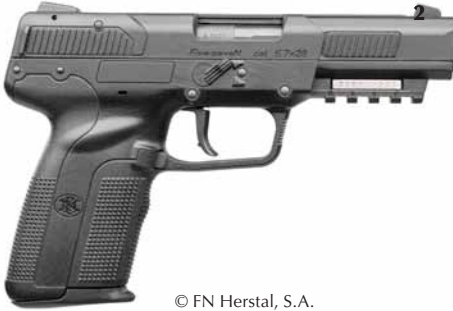
Image 3. Another example of a handgun featuring a polymer frame, the FNH five-seveN® pistol. Note the metal tag embedded in the front part of the frame, bearing the serial number.
