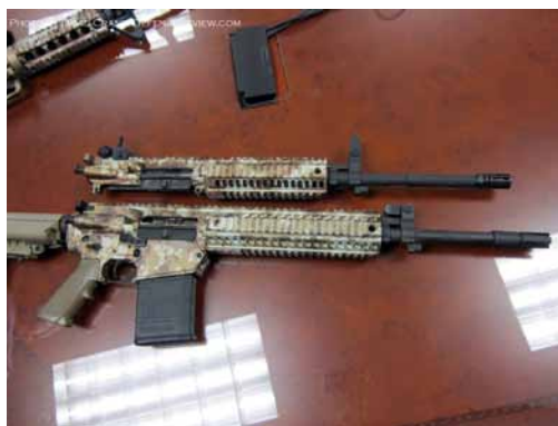
Image 7. As an example of multi-calibre approach, the CM901 features a universal lower receiver that allows calibre modularity via the swapping of the upper receiver monolithic group. This picture illustrates a 7.62 x 51 mm mounted with a 16" (40.6 cm) barrel and the 5.56 x 45 mm upper receiver (with the same 16" barrel) ready for installation.
