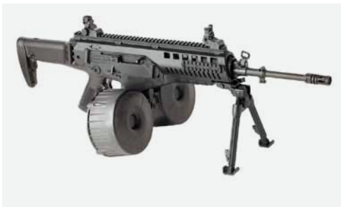
Image 6. The Beretta ARX-160A3 features a common upper-receiver approach that enables firing 5.56×45 mm and 6.8×43 mm calibres with one lower receiver, and 7.62×39 mm with a second lower receiver.
