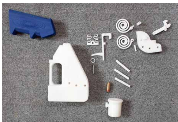
Image 2. The Defense Distrusted Liberator pistol, disassembled to show its component parts. Note the metal firing pin (nail) visible.
