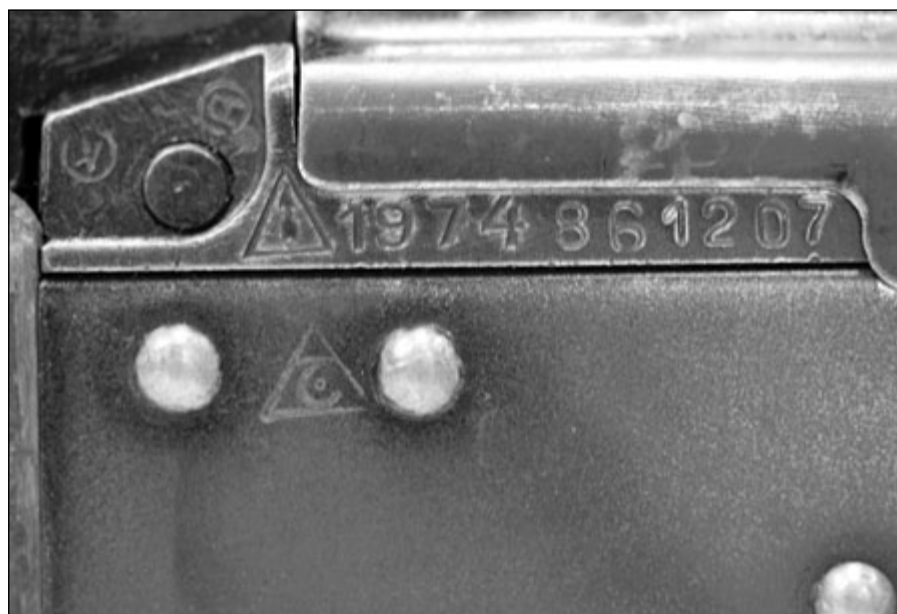
Figure 2 Iraqi import mark on a Russian-manufactured AKM
