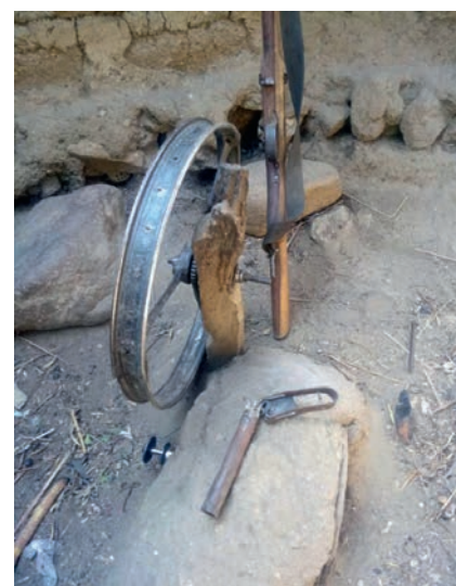
Photo 13 A muzzle-loading handgun and a simple manual furnace blower, typical of a low score on the manufacturing technology scale, location withheld, Nigeria
