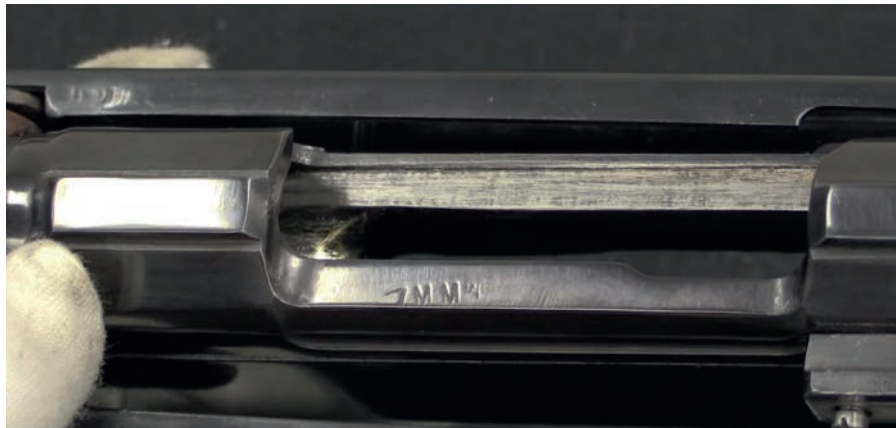
Image 3.48 A rifle with a calibre marking on the top surface of the receiver
