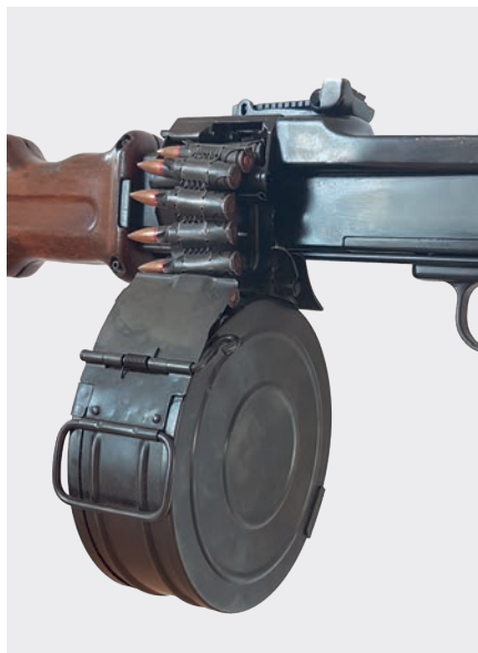
Image 3.27 A non-disintegrating belt of 7.62 × 39 mm cartridges contained within the external drum-type container of an RPD LMG
