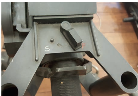
Image 5.34 Fire selector markings (S, F) on a Vektor Y3 crew-served 40 × 53SR mm automatic grenade launcher
