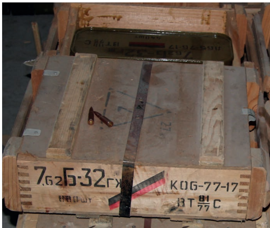
Image 4.17 Common markings on Eastern Bloc outer packaging (wooden crate)
