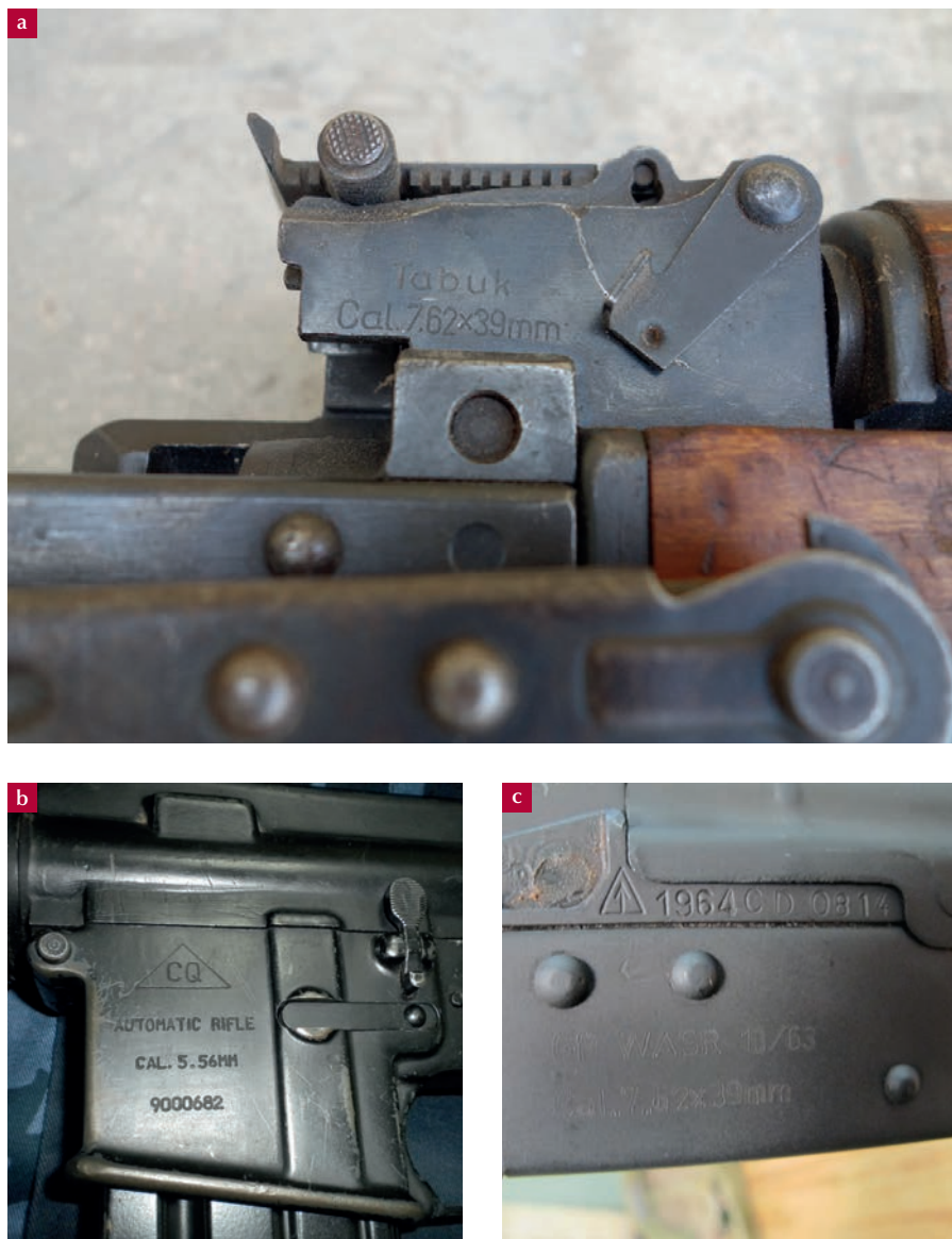
Image 3.47 Examples of model and calibre markings
