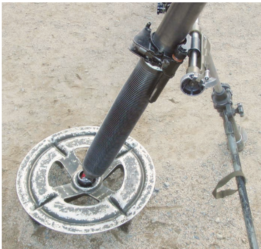
Image 5.24 The circular baseplate of a British L16 81 mm mortar
