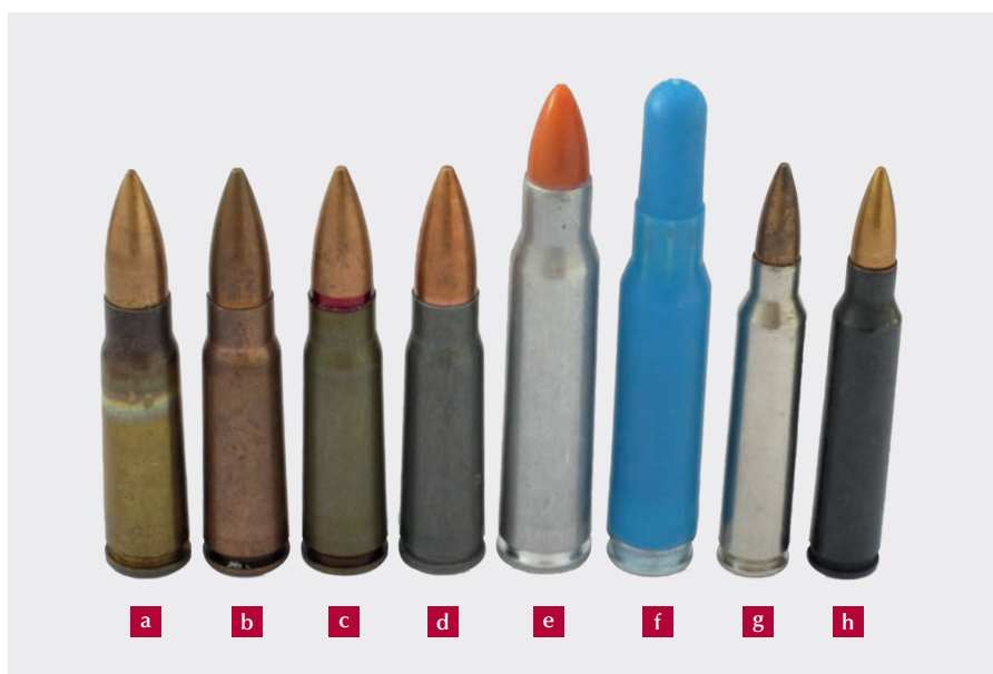
Image 4.8 Cartridges with cases made of various materials
