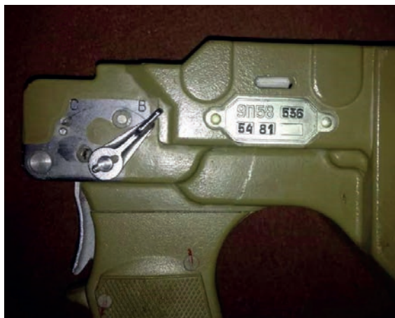
Image 5.31 Marking plate on a 9P58 gripstock for the 9K32M Strela-2M MANPADS
