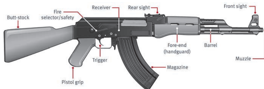
Figure 3.1 Typical features of a modern military rifle
