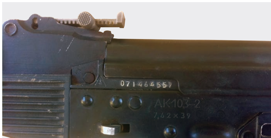
Image 3.49 Serial number marking on a Russian AK-103-2 self-loading rifle
