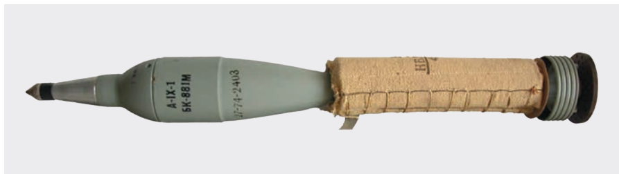
Image 5.49 Soviet BK-881M type 82 mm recoilless HEAT projectile
