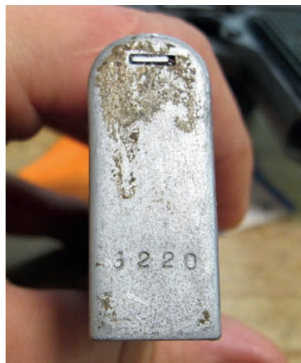
Image 3.64 Partial serial number stamped on the bottom of a Romanian TTC 7.62 × 25 mm magazine
