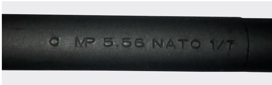
Image 3.58 Inspection marking on an M16 barrel
