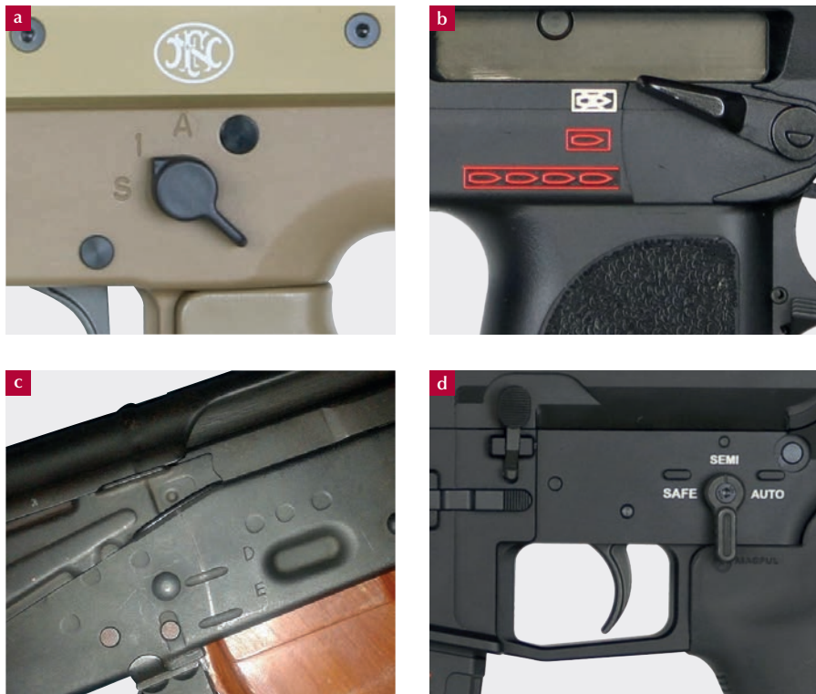
Image 3.55 Examples of safety/selector markings
