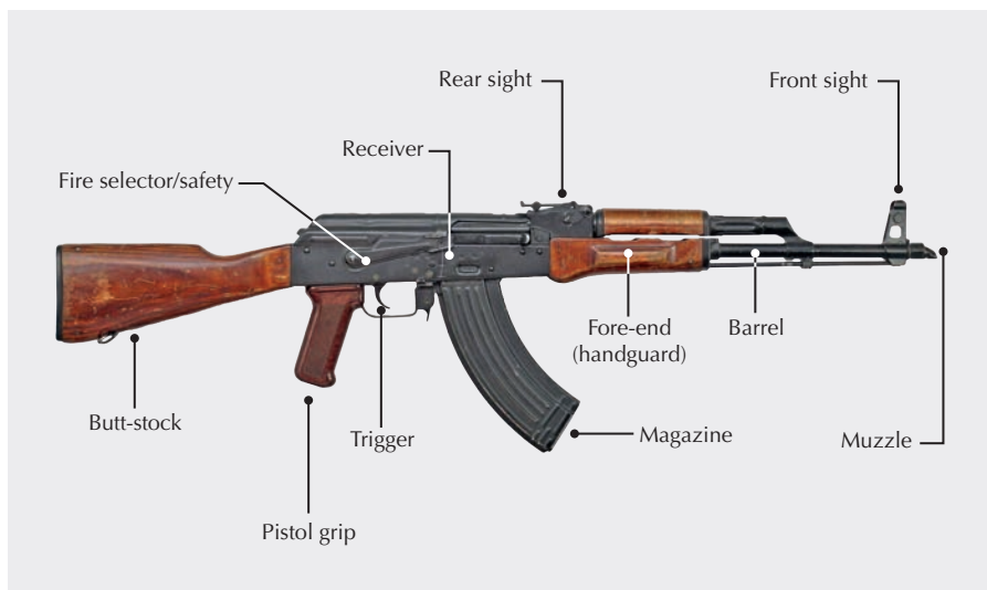
Figure 3.9 Typical features of a modern military rifle
