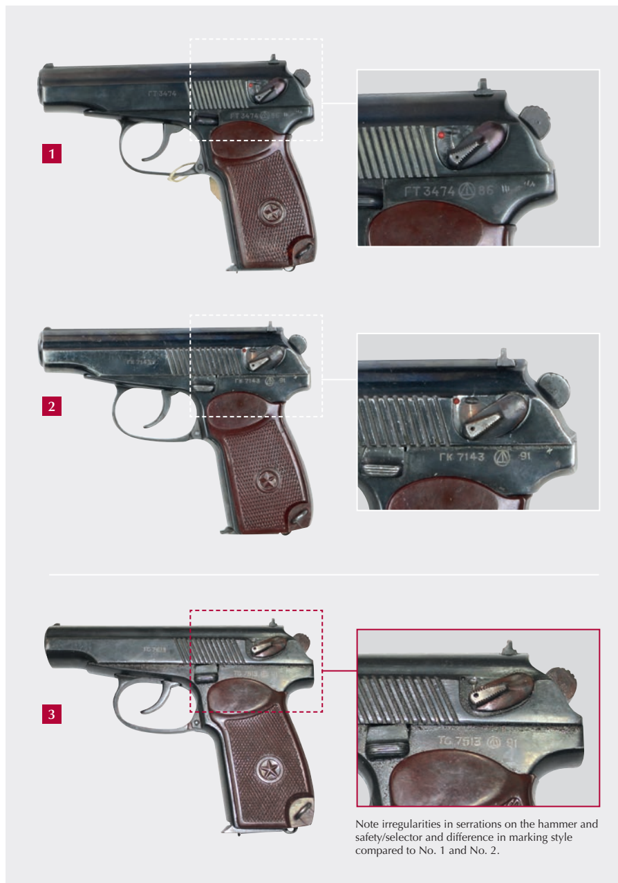
Image 6.15 Three versions of a PM-type self-loading handgun
