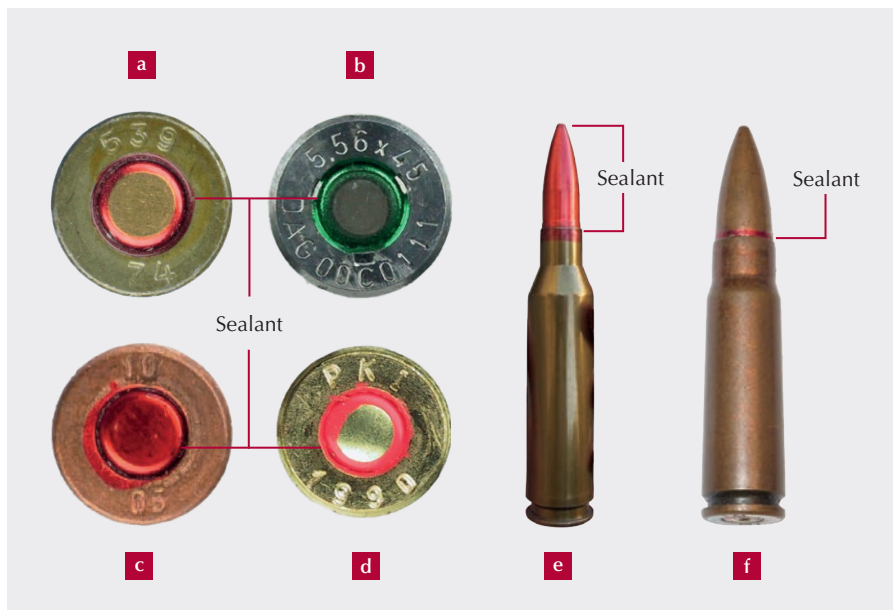
Figure 4.7 Examples of the different colours, types, and application locations of sealants
