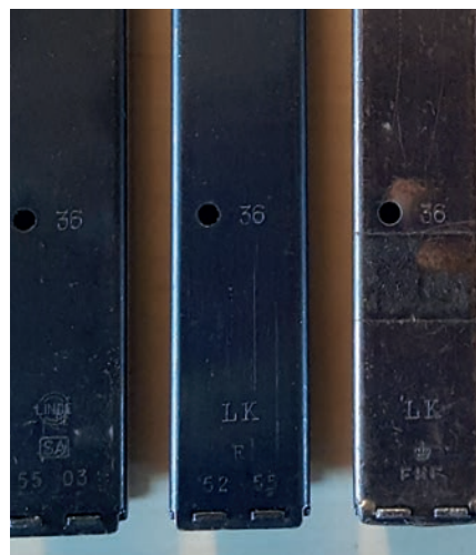
Image 3.65 Different manufacturer markings on three detachable box magazines for the Danish Hovea m/49 SMG
