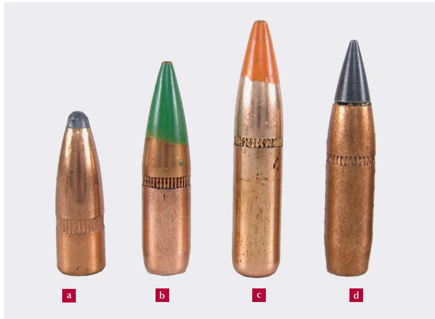
Image 4.10 Different projectiles for the 5.56 × 45 mm cartridge
