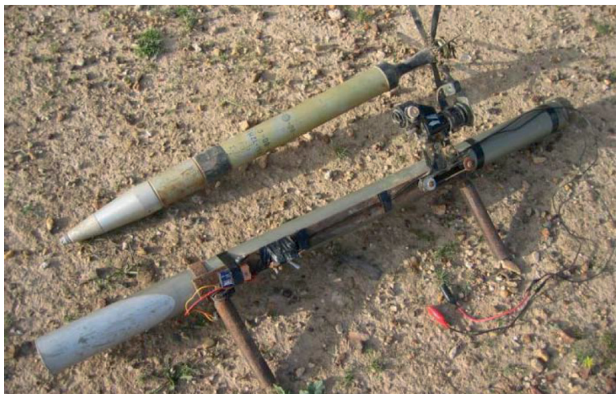
Image 6.8 A Soviet S-5 rocket (top) and an improvised shoulder-fired rocket launcher (bottom)
