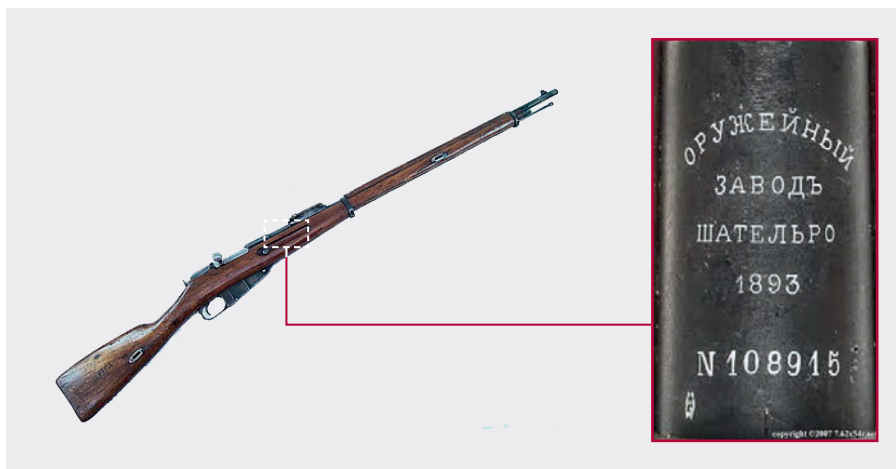
Image 3.45 A Russian Mosin Nagant rifle marked on the top of the receiver in Russian (Cyrillic script), but manufactured in Châtelleraut, France
