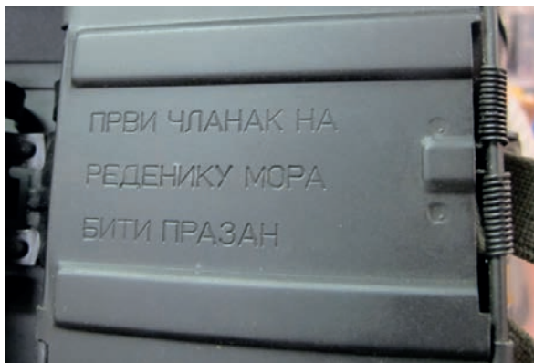
Image 5.30 A safety/operation warning marked on a Serbian Zastava M93 self-loading crew-served grenade launcher
