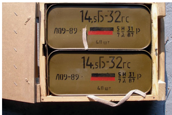
Image 5.56 External packaging crates and internal packaging tins containing Russian 14.5 × 114 mm B-32 API cartridges produced in 1989
