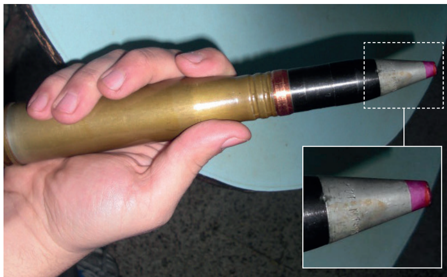
Image 5.38 A Soviet 23 × 152B mm cannon cartridge
