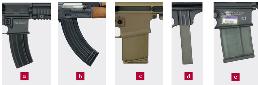
Image 3.25 Examples of detachable box magazines
