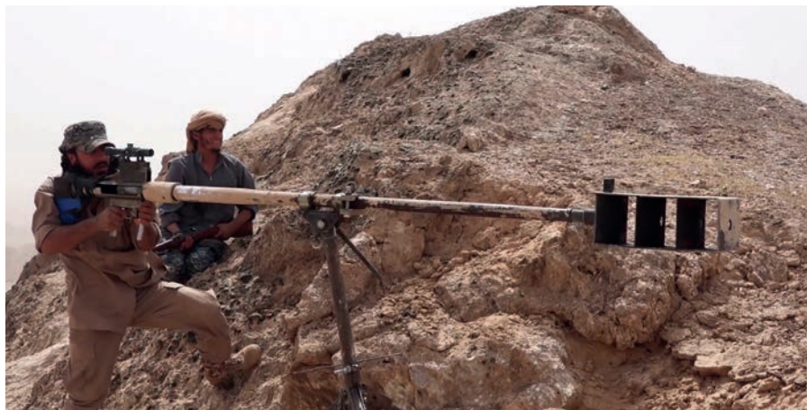
Image 6.7 A still from an Islamic State propaganda video showing a craft-produced light cannon chambered for 23 × 152B mm being used against Shia militia targets 144
