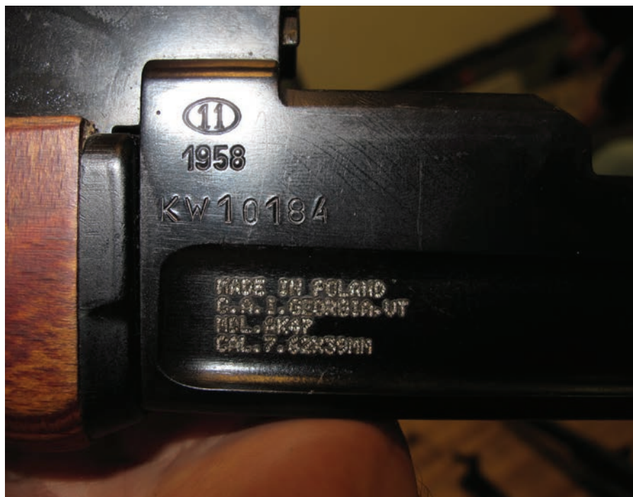
Image 3.60 Import markings on a Polish kbk AKM self-loading rifle imported into the United States
