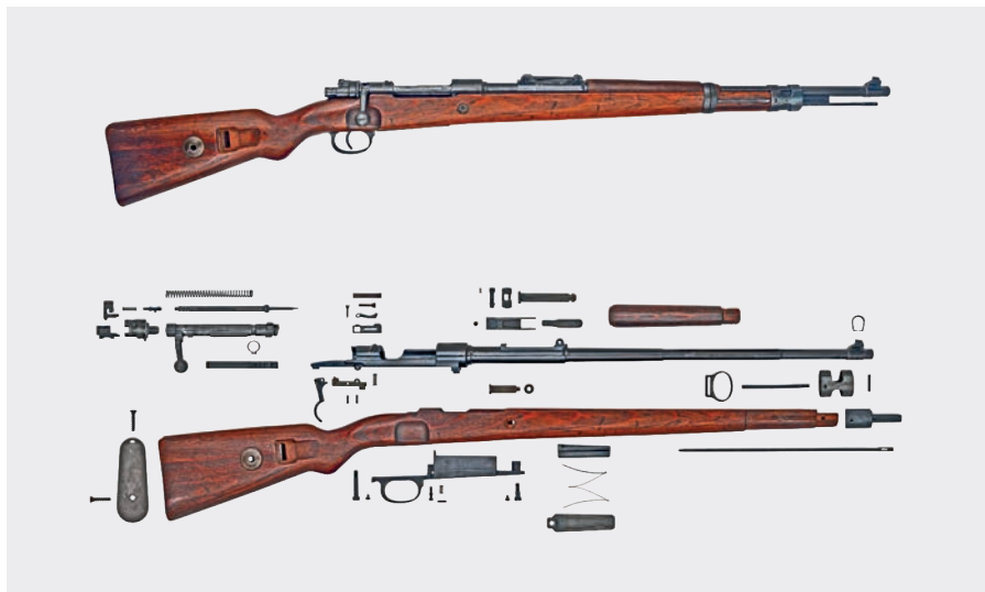
Image 3.18 A German Mauser Kar98K bolt-action rifle (top) and its component parts (bottom)
