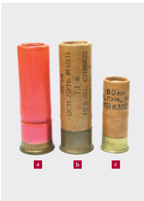
Image 5.46 Markings on various ignition cartridges
