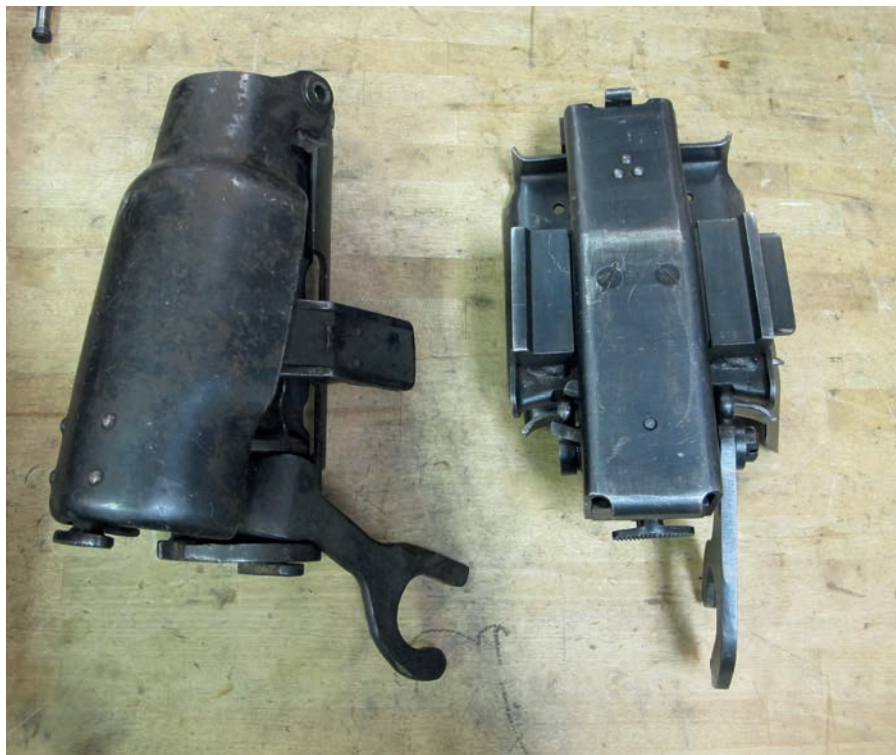
Image 3.30 The belt feed mechanisms of DShK (left) and DShKM (right) HMGs
