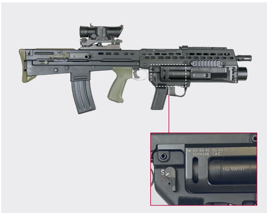
Image 3.70 Markings on a German Heckler & Koch AG SA 80 (L17A2) 40 × 46 SR mm under-barrel grenade launcher attached to an L85 series self-loading rifle
