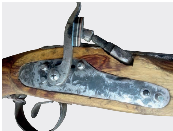
Image 6.4 A crude hand-made percussion lock mechanism fitted to a muzzleloading 'Dane gun' produced in Plateau State, Nigeria
