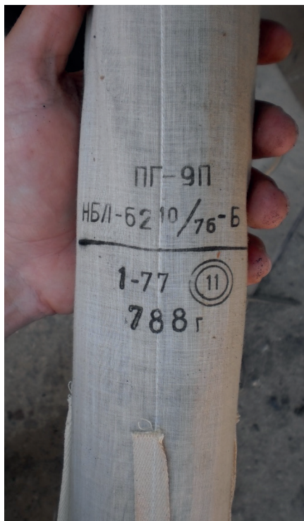
Image 5.61 Markings on a Bulgarian PG-9P expelling charge for projectiles fired from the SPG-9 recoilless gun
