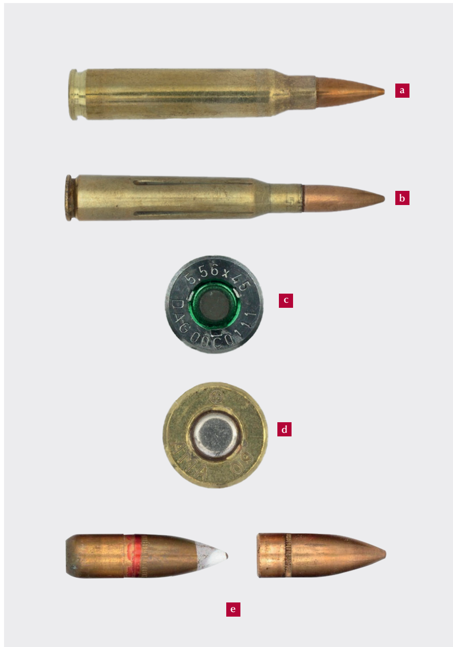
Image 4.11 Examples of various crimping, fluting, and cannelures
