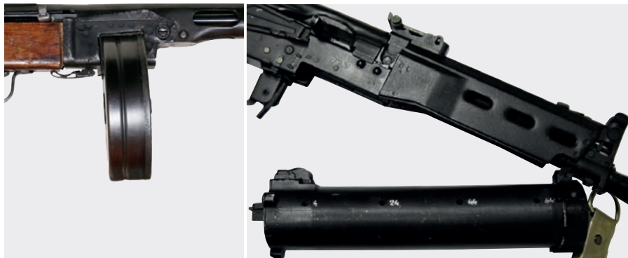
Image 3.26 Detachable drum (left) and helical drum (right) magazines
