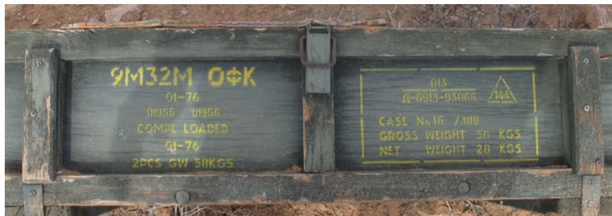
Image 5.60 Wooden outer packaging (shipping crate) containing two 9M32M type MANPADS
